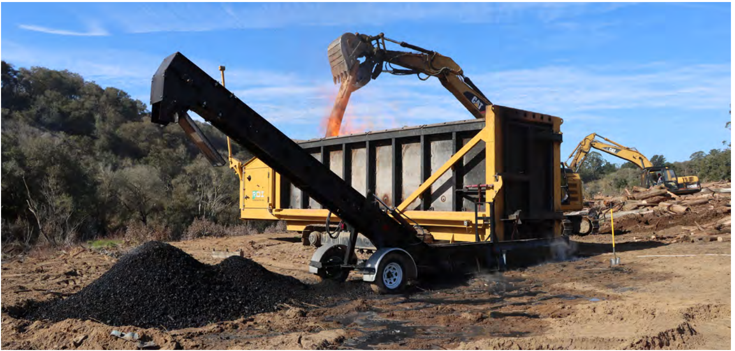
Elkhorn Slough Foundation is conducting a pilot project that uses a carbonator to process invasive eucalyptus wood and convert it into biochar as part of habitat restoration work at Elkhorn Highlands Reserve in Santa Cruz County. Photo credit: Ken Collins, Elkhorn Slough Foundation
