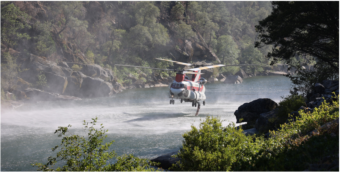
Type 1 firefighting helicopters such as the one shown here, which is being used to suppress the 2021 Dixie Fire, can carry up to 700 gallons of water and can use snorkel capabilities to refill from open water sources. Photo credit: CAL FIRE
