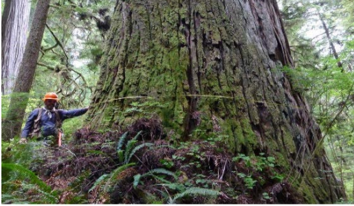
FIA plot sampling measuring diameter at breast height of a redwood in Del Norte County
