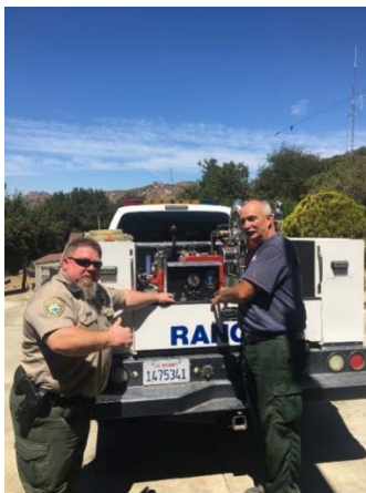
New portable water pumps installed on daily patrol vehicles in conjunction with water tanks and fire hoses allow rangers to respond to fires on patrol
