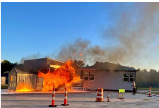
Yana Valachovic, Forest advisor, has been working with the Insurance Institute for Business and Home Safety on experiments to better understand how different building products, such as tempered glass windows, perform when exposed to fire from an adjacent building or near landscaping.
